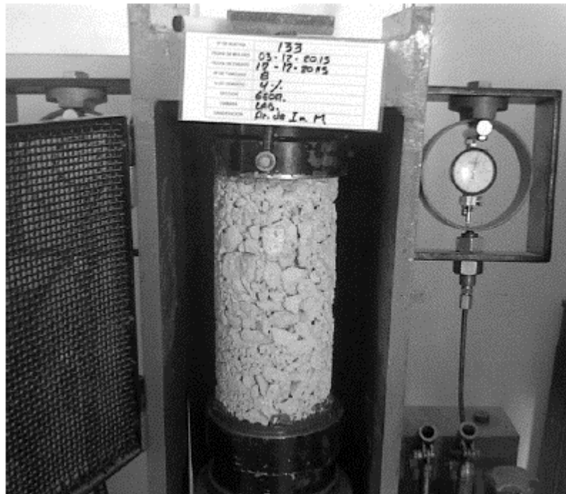
Figure 1 - Backfill specimen ready for testing in the hydraulic press
